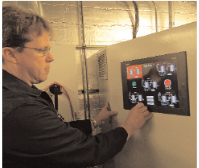
A computerized electronic system monitors both the process control and the volume of GDiesel being produced.
