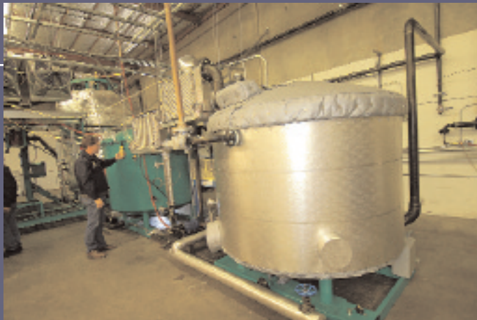
At the development center for Advanced Refining Concepts, these two tanks represent the basics of the Clear Refining process. Inside the silver tank on the right, heated diesel and natural gas are mixed and fed through a filter containing four metal catalysts. These catalysts facilitate the chemical bonding of the diesel and gas (but don’t actually become part of the fuel). The fuel then condenses and cools, running through a heat exchanger between the two tanks. The green tank holds the refined GDiesel.
